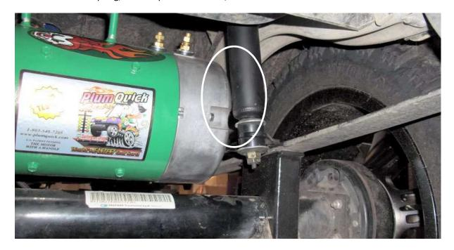
Twist the TOP shock mount plate until the bolt touches the leaf spring and tighten (torque) to manufacturer specs.
