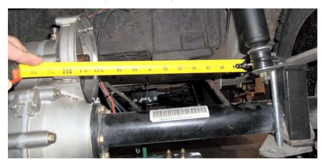
Next, removed the two shock tower mounting & spring perch bolts and slide the TOP plate back a few inches to allow clearance to install the motor.
