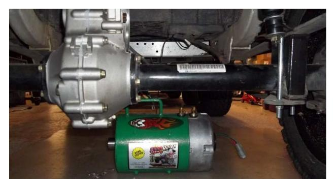
Measure between mounting face and shock tower bracket, as shown below we have 11.25", plenty to fit this motor. If the distance is too short, you may have to relive cut or grind the shock tower / leaf perch mount plate for clearance.
